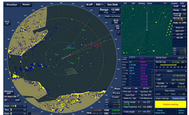
Radar picture generated from a SharpEye™ S-band transceiver with chart overlay enabled and ETD mode available on the primary or secondary PPI
